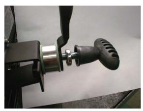
The **NEW** system is consists of a Lock Off Knob and the new lateral thrust bearing as illustrated.
