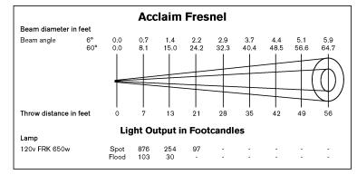
Tests conducted using a standard FRK, 650W, 120V lamp.
