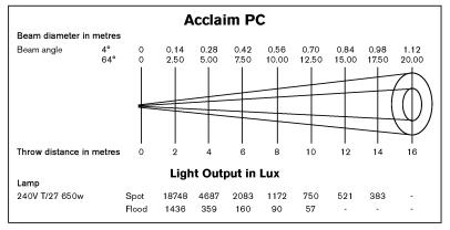
Tests conducted using a standard T27, 650W, 240V, 15,000 lumens lamp.
