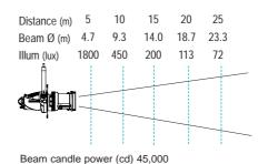
Performance at any distance: divide beam candle power by distance<sup>2</sup>
