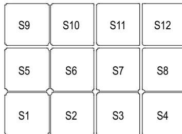
The 12 S-keys (softkeys) provide context sensitive functionality, which will assist in navigating PaletteOS software dialogue boxes and execute actions linked to the [TOOLS] and [VIEW] buttons. The amber LED will blink showing the current control when a dialogue box is open.
