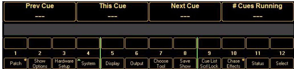
The softkey buttons are context sensitive to what you are doing. When no dialogue boxes are open, they provide additional functionality that is not available with the hard buttons on the console. When a dialogue box is open, the LEDs show you what buttons are used to jump to specific controls (lists, checkboxes, etc.). You can always see what each button will do by reading the bubbles at the bottom of the screen. The LED will blink showing you what control currently has focus.
