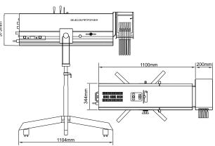
Luminaire Weight: 25.5kg Stand Weight: 9.5kg Colour Changer Weight: 2.1kg
