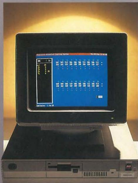
The on-screen representation of lighting cues allows the operator to recall a scene by number, check lamp position, sequence and cue timing.
