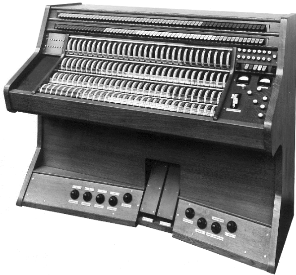
Strand system CD, two preset console, with clutch-driven resistance dimmers, Sadlers Wells, 1960s
