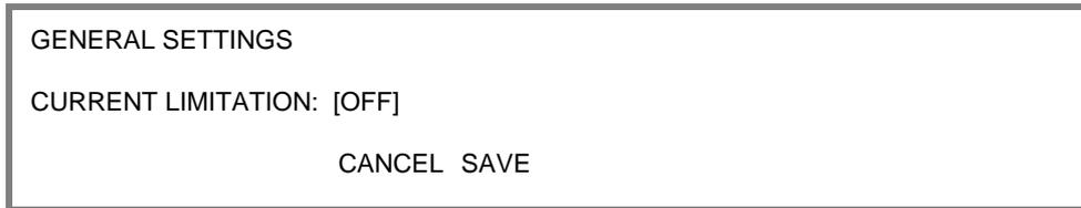
5. Press EDIT and using the encoder wheel, choose ON or OFF to enable or disable the current limitation.
