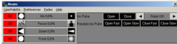
MAC 2000 beam control with iris pulse control
