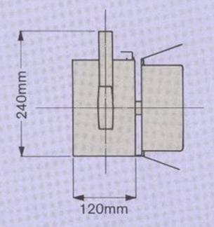
A floodlight with a high intensity fixed beam angle giving an even wash of light and fitted with integral external shutters to control light spill and beam shaping.
