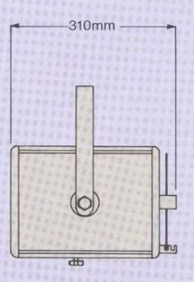
A compact spotlight producing a soft edge to the light beam with a variable beam angle.
