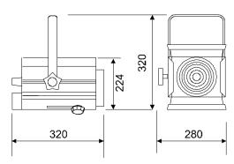
Weight: 4.6 Kg Packed Weight: 6.1Kg Carton Size: 275 x 250 x 380 Carton Size Cubic: 0.026
