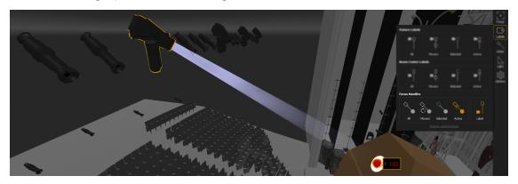
Focus Handles create a controllable point at the end of the beam of an automated fixture, which can be dragged to focus a single fixture, or multiple fixtures together while maintaining their spatial relationships.
