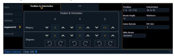
Under the Augment3d section in Patch, fixtures have fields for XYZ Position & Orientation. You can also enter information for Beam Angle, Shutters, and Gobo Rotation.
