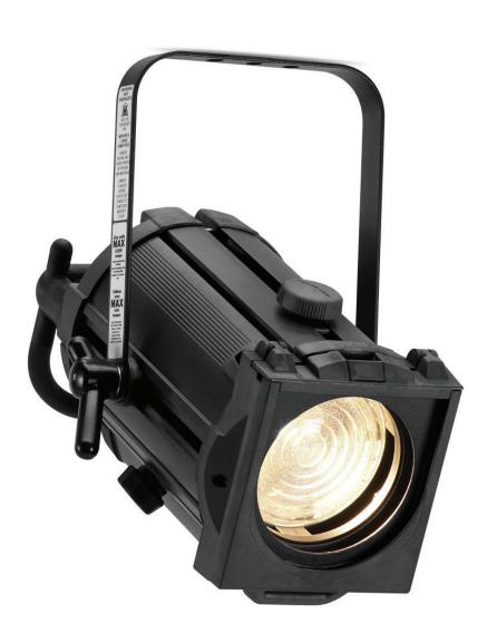
The Acclaim 6°-60° Fresnel is a 300W / 575W / 650W general purpose Fresnel ( $4\frac{1}{4}$ " diameter lens) for theatre, small studio and display lighting applications which produces an adjustable cone of light with a soft edge that is easily blended with adjacent beams to provide even illumination.
