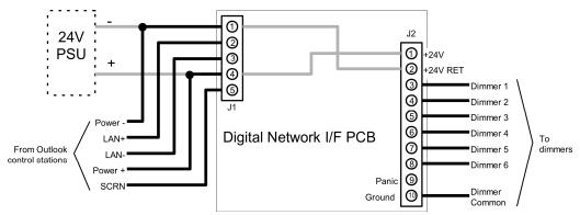
4 Connect up to six analogue input dimmers, or other similar devices to J2, as shown above.
