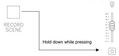
All LEDs will flash momentarily. When recorded, the LED above the selected fader will light up.
