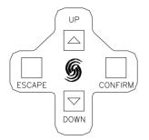
Basic navigation for the 301 is done with four buttons (represented to the left). The functions of the keys are labeled on the bottom line of the LCD screen. Escape on the left, Confirm on the right and Up / Down in the center separated by a slash (/). With the example below, Escape = Quit, Up/Down scroll through options 1, 2 and 3. Confirm = Confirm.
