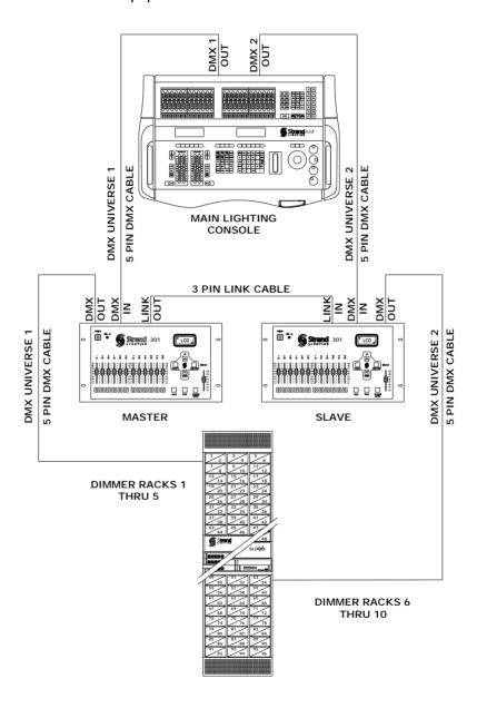
Connect a 3 pin cable to the link input of the master 301 console and connect it to the link output of the slave 301 console.
