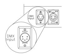
Plug a DMX512 cable from the main lighting console's first DMX output to the DMX512 input of the 301.
