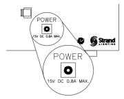
Plug the appropriate power adaptor into the console where shown. Plug the male end into the appropriate electrical service.
