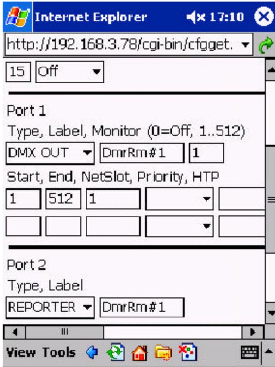
This graphic illustrates how easy it is to route DMX using a simple point and click web browser interface and is the most powerful part of a ShowNet network. Over 18,000 DMX addresses are supported on all Strand Networks.
