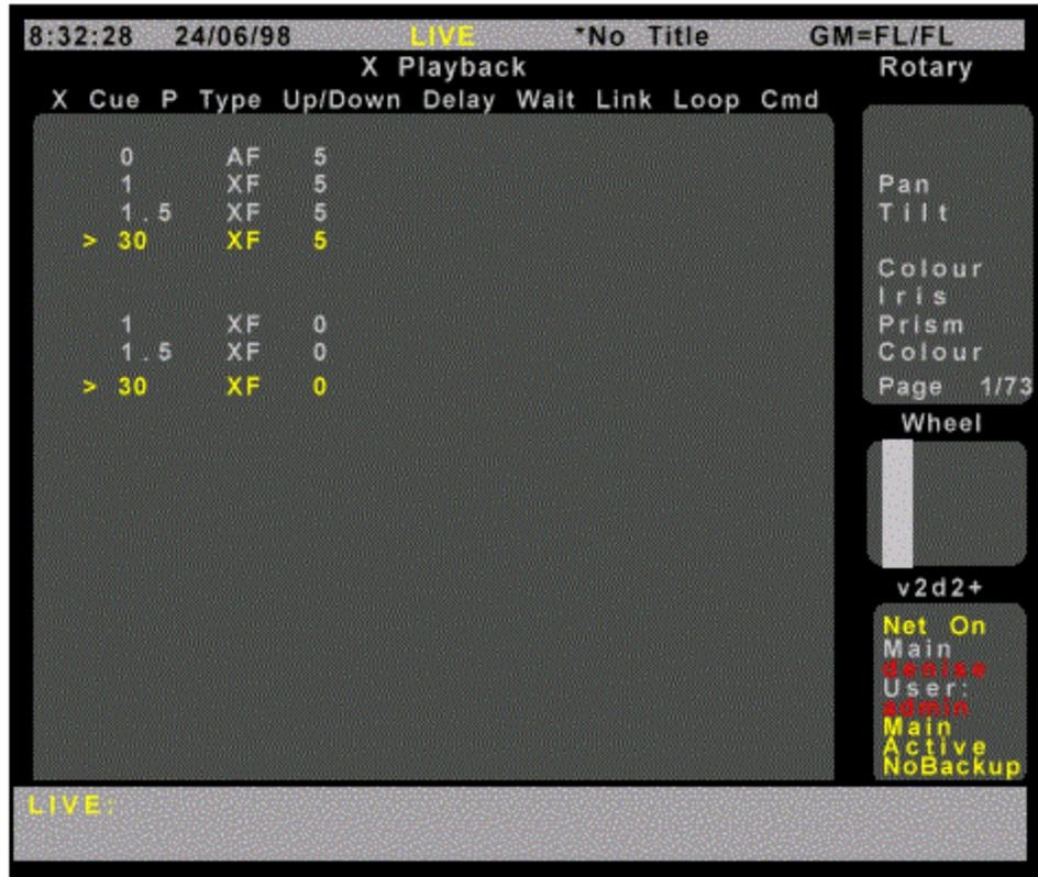
This window is mainly used when running the playback. Each playback has a title line followed by completed or currently running cues. This is followed by a blank line and then all unrun cues. The last recorded cue is shown at the bottom in all red. This disappears when the console is switched off and on again, or when it is disabled in the User Setup Screen by turning the [Show Last Recorded Cue](#) field to **OFF**.
