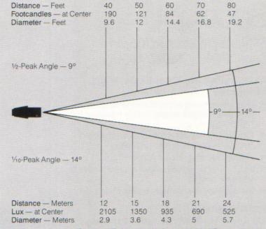
Performance at Any Distance: Footcandles or Lux = 303,500/Distance<sup>2</sup> Diameter = Distance x .24
