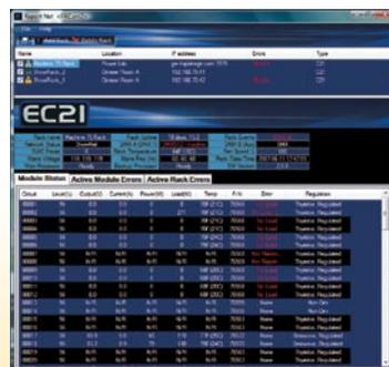
*Report.net, Strand's new Windows-based monitoring software, supports all of Strand's dimming systems. Configuration and status reporting for large integrated systems can be viewed on a single display.*
