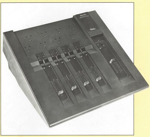
The sculptured form of the new Micro 8 is far removed from the traditional, somewhat utilitarian image of a stage lighting dimmerboard but this table-top console really is a self-contained, highly portable lighting control. The contoured surface is not just futuristic styling but is truly functional as it guides the user's eyes and fingers so that he, or she, can concentrate on the resulting lighting composition.
