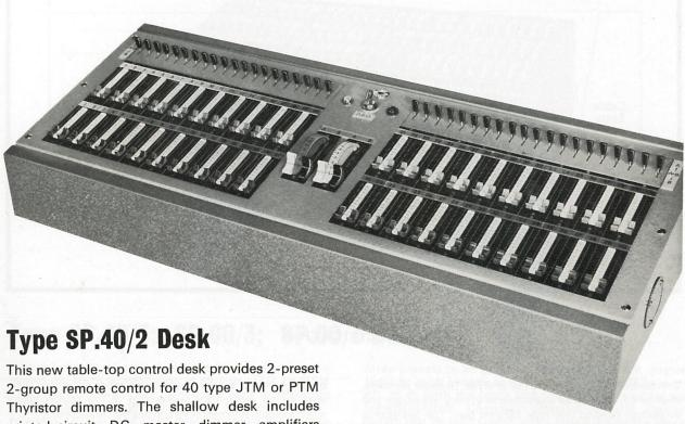
This new table-top control desk provides 2-preset 2-group remote control for 40 type JTM or PTM Thyristor dimmers. The shallow desk includes printed-circuit DC master dimmer amplifiers which previously have only been used in our larger and more expensive lighting controls; these amplifiers allow the four master faders to have an effortless, fingertip motion.
