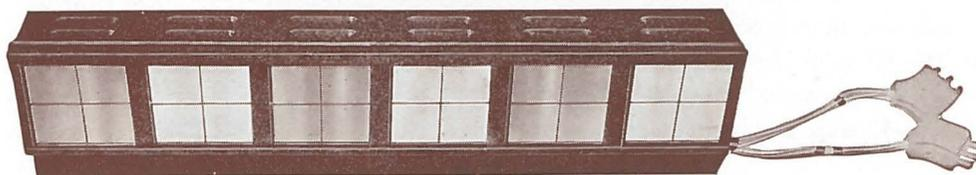
This magazine equipment is designed to be as compact and light in weight as possible in order that it may hang vertically or horizontally on framed scenery. The light dispersion is wide, particularly in the double sided model, free from hot spot, making it particularly suitable for lighting window and door backings. In small stages it will also be useful as footlight or as groundrow to light the bottom of cycloramas and backcloths at close range.
