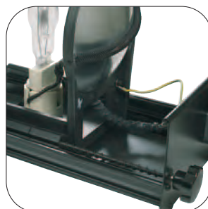
Focus adjustment by an endless screw mechanism
