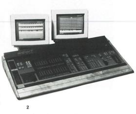
ules and control up to 1,000 independent dimmers. Two types of performance modules were offered — a cross fade unit that progressed through cues in sequence, and a mixer unit with four controls for mixing and balancing memories. Two decisions were made, essential to the mode of operation, which distinguish the AVAB range from other designs. The outputs from the cross fade units and mixers combine with "highest precedence" logic, and control button operating sequences
