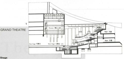
Proscenium - 15m (w) x 9m (h) x 19m (d); Stage lighting bridge and tower panels can adjust opening to a minimum of
