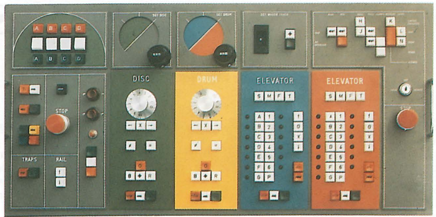
Drum Revolve control panel.
