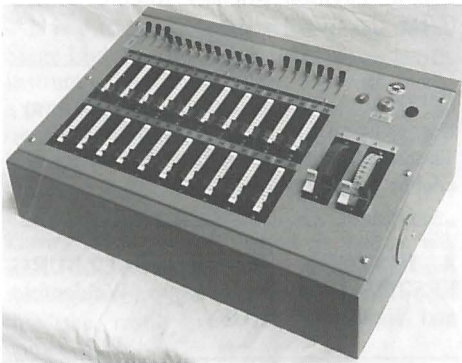
S.P. Desk. (Earlier models had quadrant faders and groupong switches that became known as flying buttons )
