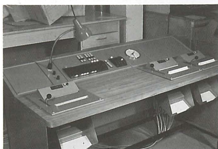
Memo-Q desk with three punch-card readers for presetting (made by Grossmann and marketed by Strand in the early 1970s)
