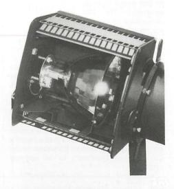
reflector, maximise efficiency in terms of usable light collection. A novel system for moving the reflector control from peak centre beam to flat field, without the need to readjust lamp orientation. As far as is known, this is the only profile luminaire which gives beam quality adjustment without the need to adjust the lamp alignment.
