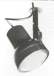
for PAR 46 and 56 lamps. The technical data for the PAR 46 (shown here) is: Input voltage 220-240V Output 5.5V, Watts 25. The fitting can be supplied ready to accept a standard hook clamp for 48mm bars or for direct attachment to a 'besa' box. Its standard colour is black but other colours are available to special order.
