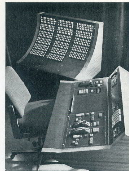
System DDM and its computer below. This particular model is the 240 channel model for the Adelaide Festival Theatre, Australia.
