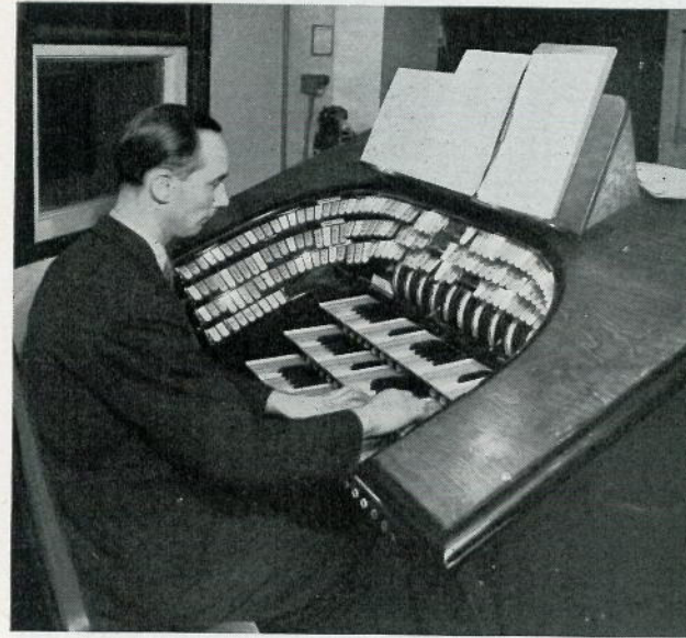
Drury Lane Theatre, London, 216 channel Light Console.
