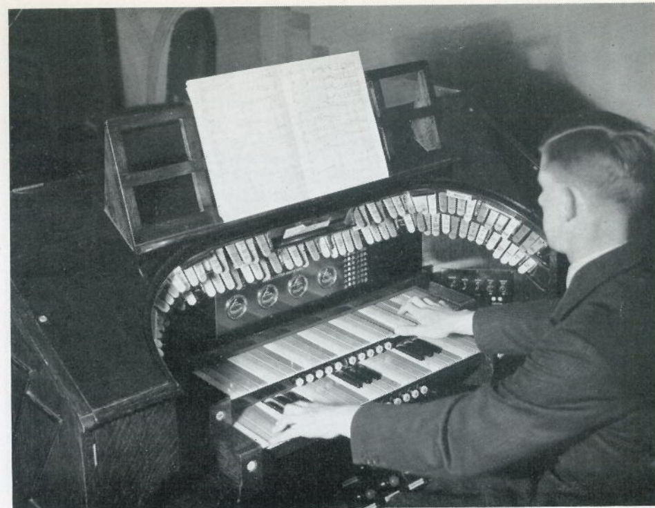
1935. Youth playing the Strand Light Console. The semi-circular rows of stop keys select the dimmer channels for operation from the master keyboards. Memory group selection is by piston under each keyboard.
