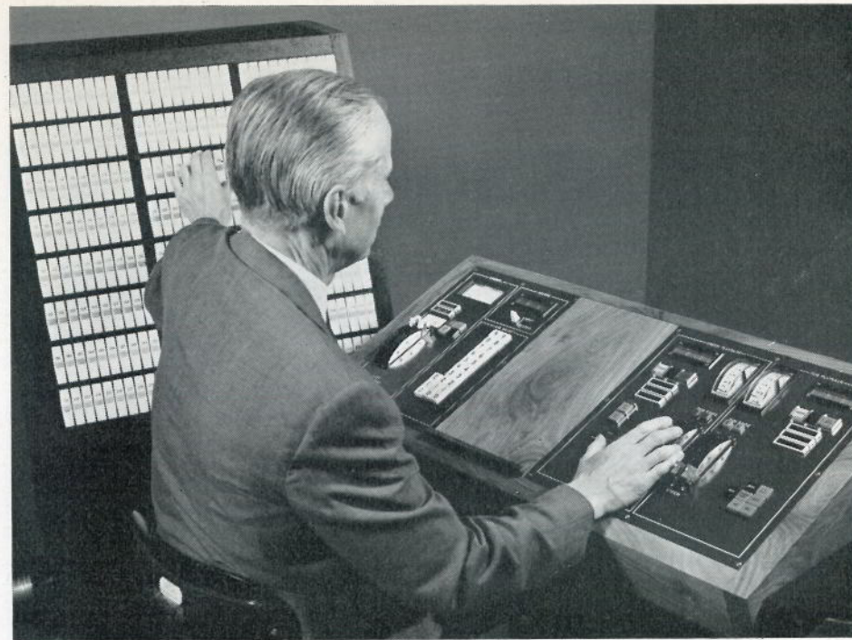
1971. Veteran playing the Rank Strand lovable computer. Individual rocker tablet controls for 240 channels are on the wing. Dimmer memory controls and numerical selector to break sequence is on the left of the desk and the playback controls on the right.
