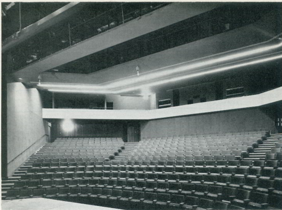
Shaw Theatre, Camden. Auditorium showing lighting bridges overhead. Balcony contains the boxes, projection and control rooms.
