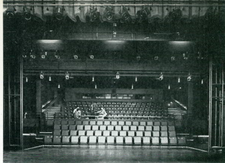
Gulbenkian Centre University of Hull: View of theatre arranged for proscenium type production. The fixed seating area has been brought into service with movable seating tiers in front and the floor opened up for the first rows. The proscenium is formed by the periaktoi units.
