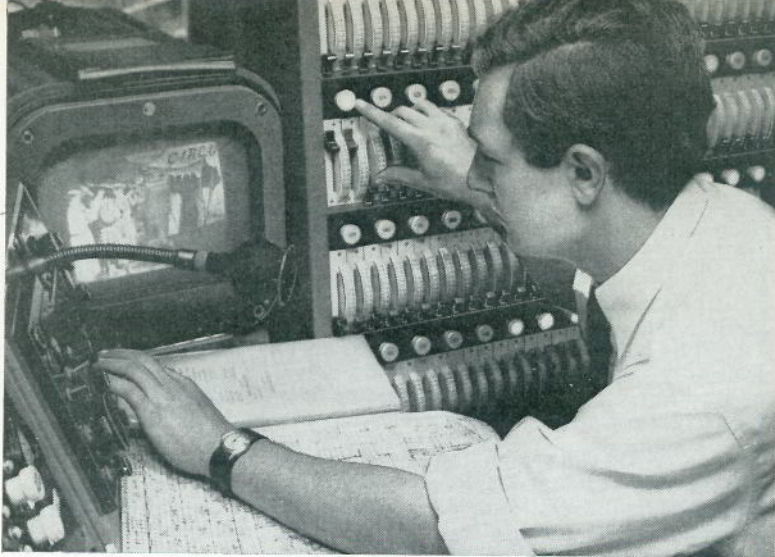
Where it all started. BBC Riverside Television Studios. Lighting Supervisor using Strand system C control. (Photo by courtesy BBC.) The two Riverside Studios were pilots which determined the form those in the T|V centre were later to take.
