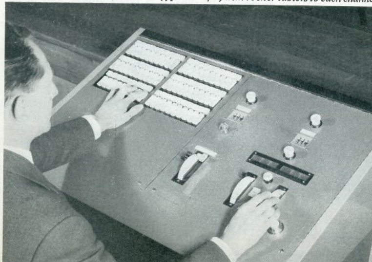
Instant Dimmer Memory Console (type IDM|R) with rocker tablets to each channel.
