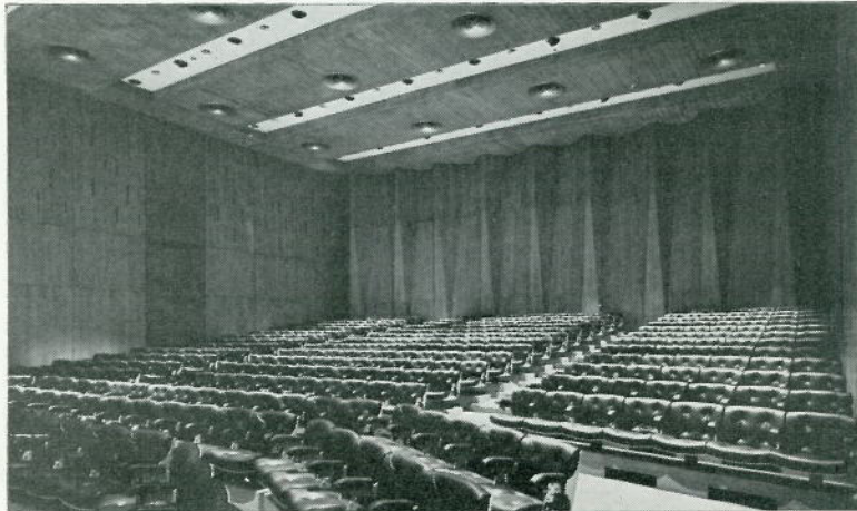
Purcell Hall. Concealed spot lighting apertures are set in the strips of white in the concrete ceiling. The large circular fitments are for ventilation.
