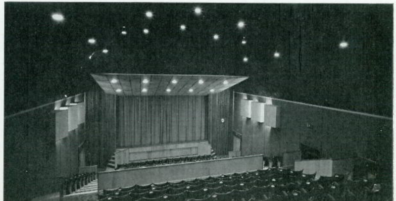
Rotherham, Civic (1960) Hadfield, Cawkwell and Davidson. Consultant: Percy Corry. Civic theatre for amateurs and professionals. Chapel purchased and converted. 387 seats in one tier. Pros. 26 ft. wide by 14 ft. high. (24 ft. 6 in. to RSJs above stage). Removable forestage/orchestra pit. Cost £40,000. (TABS 23, ii)
