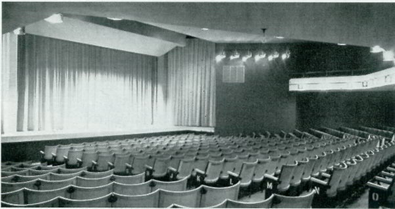
Corby Civic Theatre (1965) Enrico de Piero and Partners Amateur/Professional. 545 seats in two tiers. Pros. 26 ft. x 14 ft. Stage depth 29 ft. plus 5 ft. apron. Overall width 58 ft. Height to grid 28 ft. Situated under multi-purpose assembly hall seating 1,388 used for concerts, dances and wrestling. The foyers are also intended for exhibitions. (First Review)
