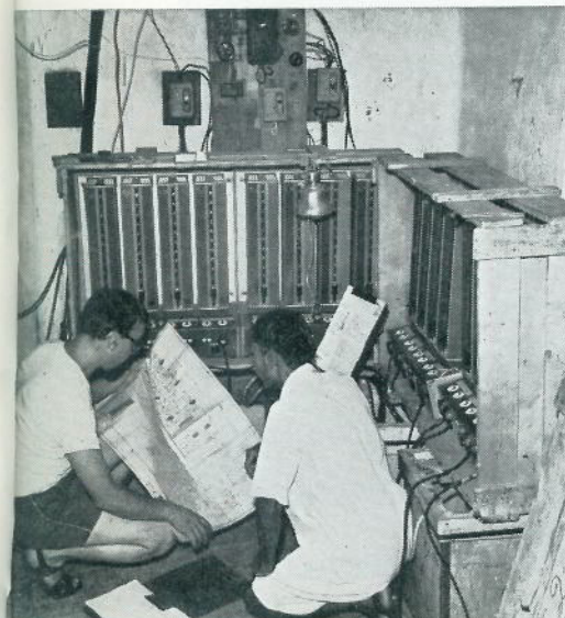
Four Junior 8 boards, packed to travel and operate in two crates.
