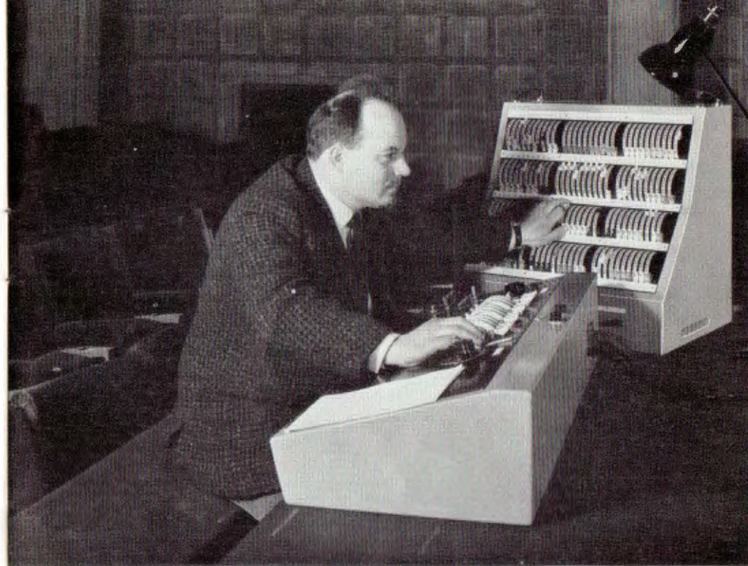
Fig. 1. Francis Reid at the portable control position in the stalls. 120 dimmer channels on his left and full set of master controls on his right.
