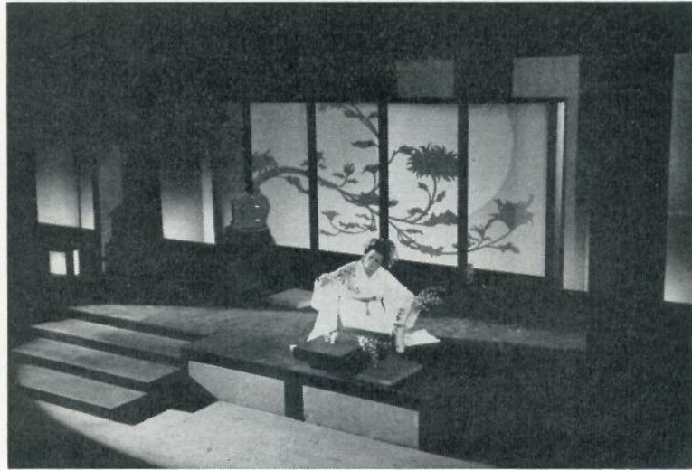
FIG. 2. Close-up of the platform island for Butterfly with translucent screen panels. The scene is the interior of Butterfly's house with a night garden beyond. The garden pattern is by Direct Beam projection.
