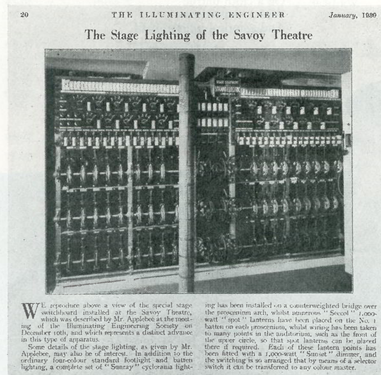
Description of the old 1929 stage switchboard at the Savoy from "The Illuminating Engineer" of January, 1930.
