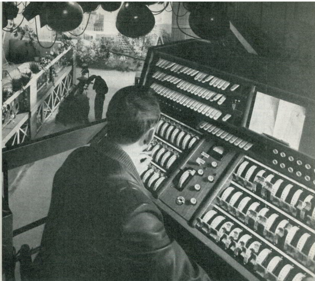
View of new Cologne Television Studio showing operator at the Strand lighting control with a scene set in the background.
