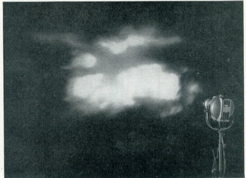
Hand painted cloud slide on mica projected from a Pattern 23W Spot ten feet from the skylcloth.
