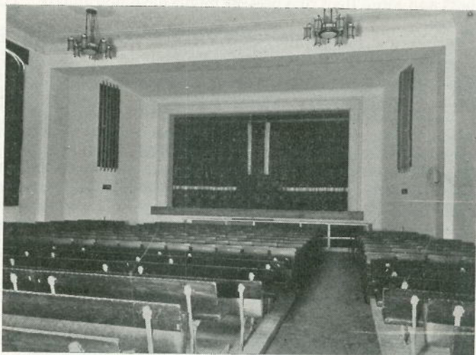
Fig. 1. THE AUDITORIUM LOOKING TOWARDS THE STAGE The rear rows of seats are on tiered removable platforms as the floor is flat, the Hall sometimes being used for Dances, etc.
