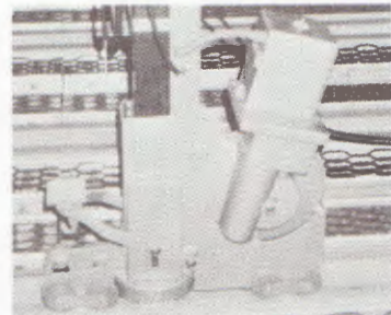
A motorised telescope photographed on the slotted grid of a modern TV studio.
