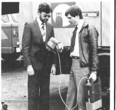
The Arri Report 200 Watt H.M.I. Note the combined buffer unit, ballast and battery pack.
