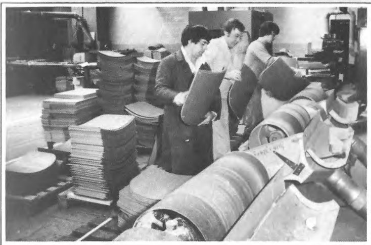
Drum sanding new plywood seat backs. ▼
