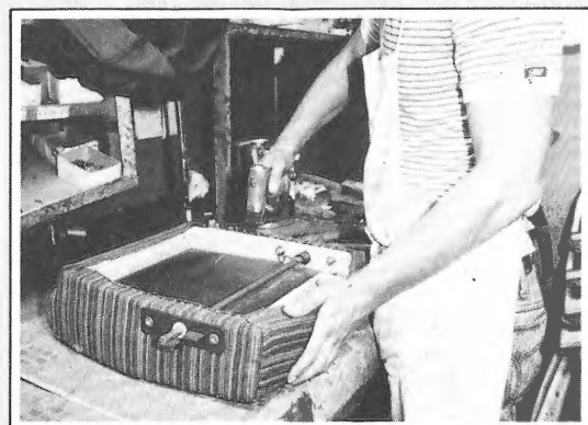
Using a compressed air stapler to fix a seat cover. ▼
