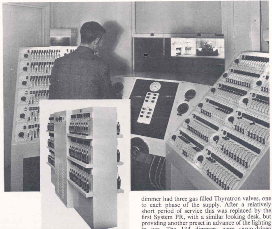
The Circuit Fault Mimic Panel laid out to correspond to the geographical position of the socket outlets in the theatre. Each channel is colour coded to show its phase and a red light indicates any channel which is alive but not lighting. There are also clear master warning signs to draw the operator's attention to circuit faults and overload conditions.
