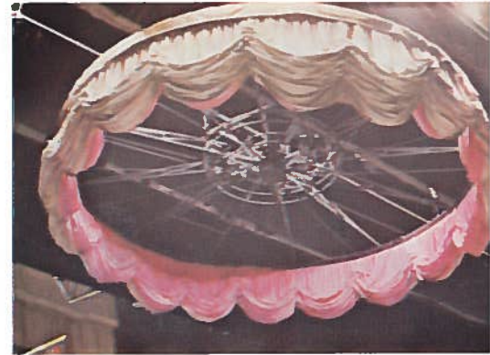
Finale. Circular track which revolves, opens to semi-circle, and festoons up to 25 ft. in height, yet flies in depth of only 2 ft.
